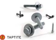
Taptite is trilobular (triangular shaped) fastener that forms its own thread when driven into a material during assembly. This eliminates stages in the assembly process such as pre-threading and degreasing. This technology leads to significant productivity increases. Taptite is used frequently in engine applications.
