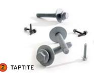
Taptite is trilobular (triangular shaped) fastener that forms its own thread when driven into a material during assembly. This eliminates stages in the assembly process such as pre-threading and degreasing. This technology leads to significant productivity increases. Taptite is used frequently in engine applications.
