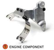
Several of our products comprise both stamped and die-cast components that are joined to make a more complex product. The product in the picture is a catalyst console that is made of sheet metal, aluminium, fasteners and other components supplied by sub-suppliers.
